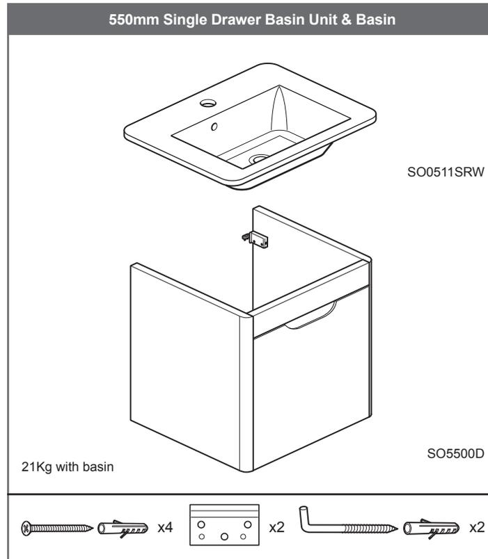
**Tools & equipment needed:** Drill, 8mm Suitable drill bit, Phillips screwdriver, Spirit level, Ruler/tape measure, Pencil, Silicone sealant (clear).
